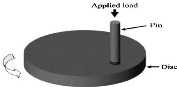
**Fig.1 schematic diagram of pin on disc wear tester**
