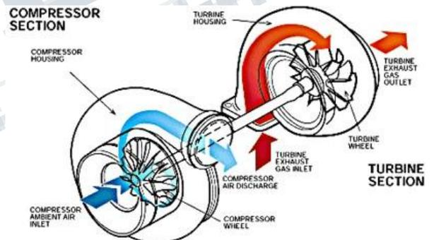
**Figure 3 Working of Turbo Charger**
