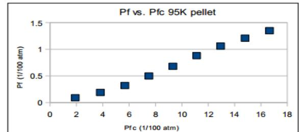
**Table 4 Adsorption Isotherm for Zeolite 13X**
