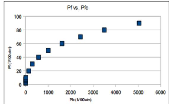
**Table 3 Adsorption Isotherm for Zeolite 5A**
