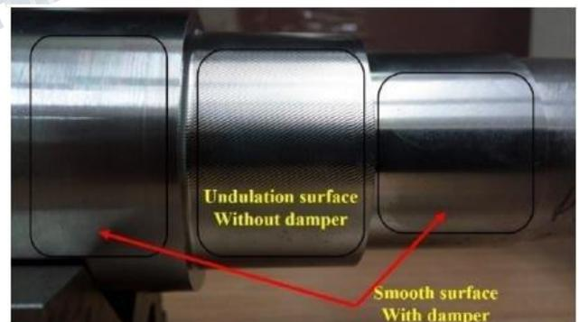
**Figure 12: Effect of damper in improving the surface finish**
