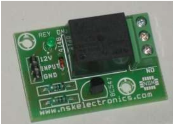
This Board can be used to Control Solenoids, Motors etc.
