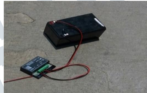
Fig.9 battery and charge controller
