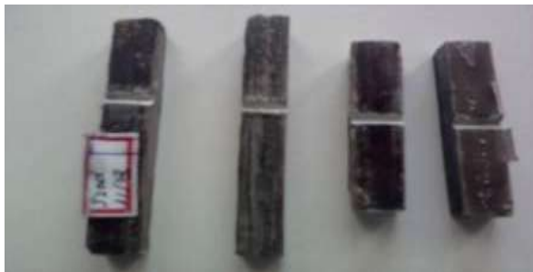
Fig 3.4: Prepared tensile and impact test Specimens
