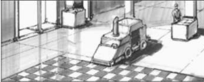
Design of robot for automatic tile installation
