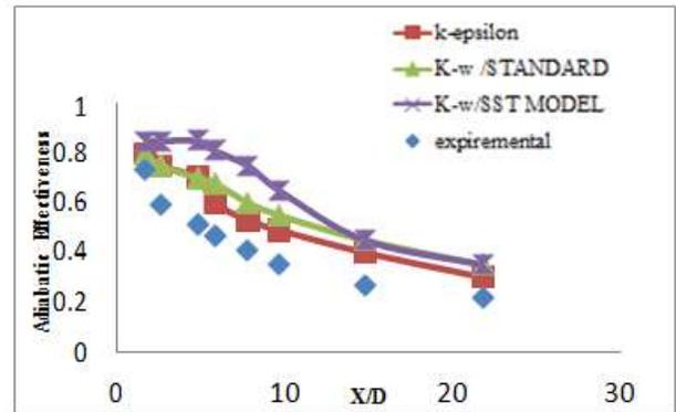
**Fig.4 Comparison of experimental and CFD film effectiveness (centerline) for cylindrical hole model**
