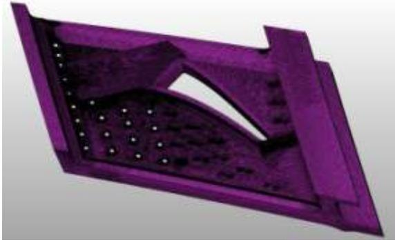
**Fig.9 Top platform model meshing**
