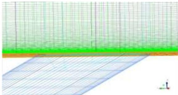
**Fig.2.1 Fine mesh near the bottom wall of mainstream domain**
