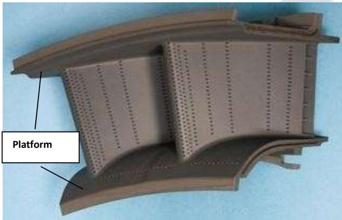
*Fig.6 Nozzle guide vane*
