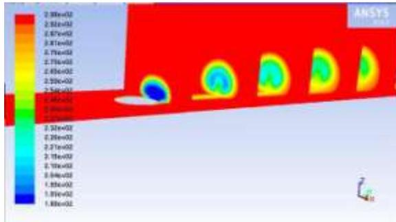
**Model 3: SST  $k-\omega$  turbulence model
