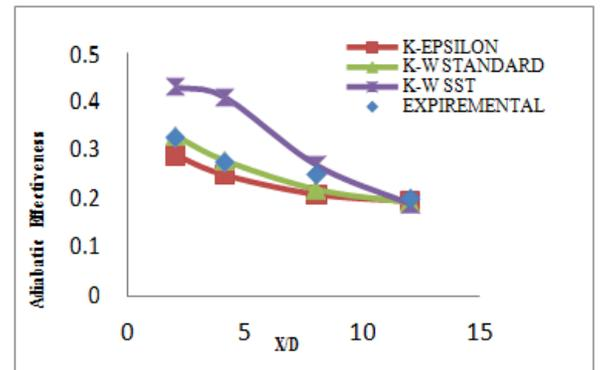
**Fig.5 Comparison of experimental and CFD film effectiveness (spanwise) for cylindrical hole model**
