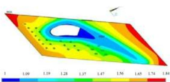
**Fig.12 Considering Impingement cooling and film cooling**
