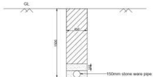
Fig 2. Cross section for pipeline excavation
