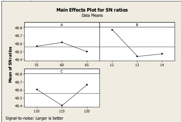
**Fig.5: Main Effects Plot for Hardness**
