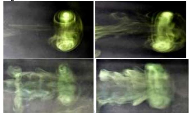
**Figure 2: Vortex rings generated at different stroke ratios, a)1, b)3, c)4 and d)5**
