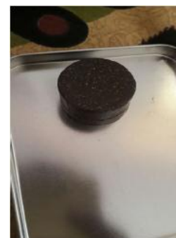
Figure. 11. View of 80%ldpe 20%husk (percentage by weight)
