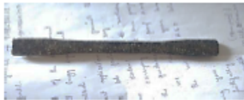
Figure. 13. Tensile specimen of 80% LDPE and 20% SSH
