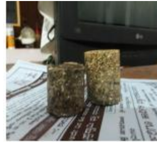
Figure. 8. LHS 70%ldpe 30%huskpowder, RHS 60% ldpe 40% unpowdered husk (percentage by weight)
