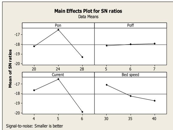
**Fig. 4. Main effects plot for Electrode Wear**
