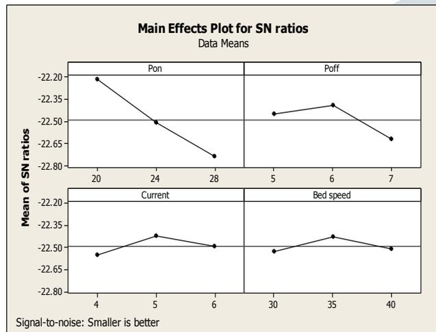
**Fig. 2. Main effects plot for Surface Roughness (Ra)**
