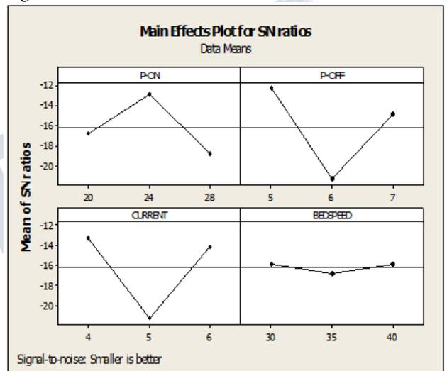
**Fig. 3. Main effects plot for Dimensional Accuracy**
