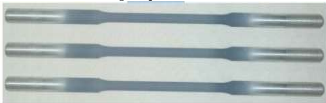
Aluminium A319 Fatigue Specimens coated with Alumina-Titania
