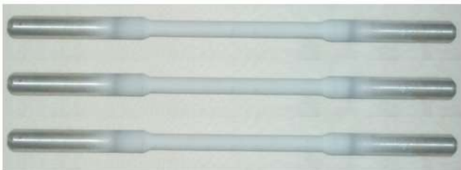
Aluminium A319 Fatigue Specimens coated with Zirconium
