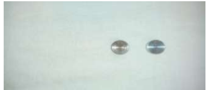
EN19 & A319 Reference Wear test Specimens
