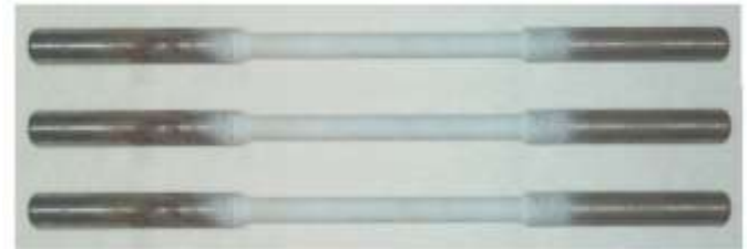
MS EN19 Fatigue Specimens coated with Zirconium
