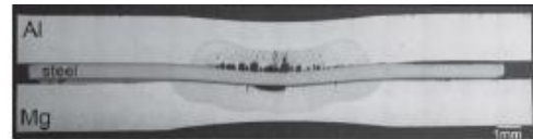
Fig. 17— Typical Al/Mg weld made with a Zn coated steel interlayer and 28kA welding current.
