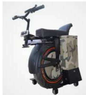
Fig.7 Assembled view of Single wheeled electric bike (Prototype).
