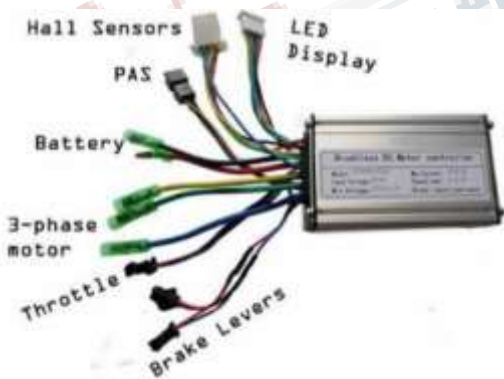
Fig.4 48v Electric controller with all the terminal ends.
