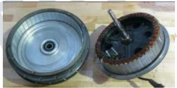
Fig.6 Schematic representation of a DC Hub Motor with two side coverings.
