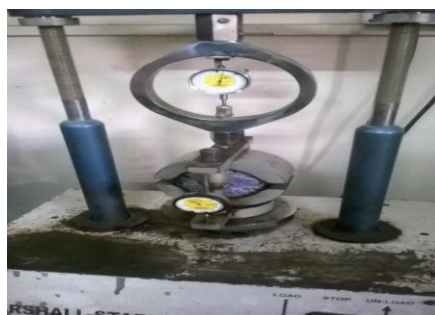
Fig 4. Marshall Stability Test in Progress
