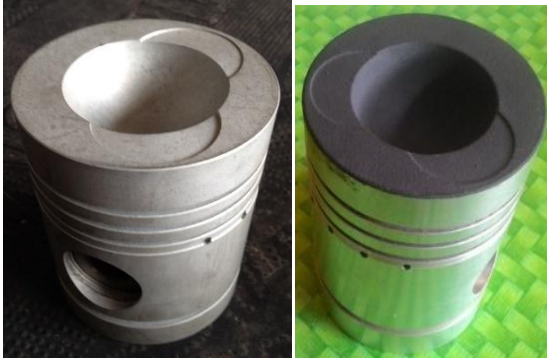
Fig.3. Pistons before and after coating with TiO 2 powder
