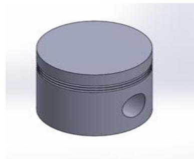
**Fig 4.1: Isometric view of piston**
