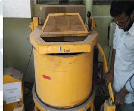
**Fig.3. Pan concrete mixer.**
