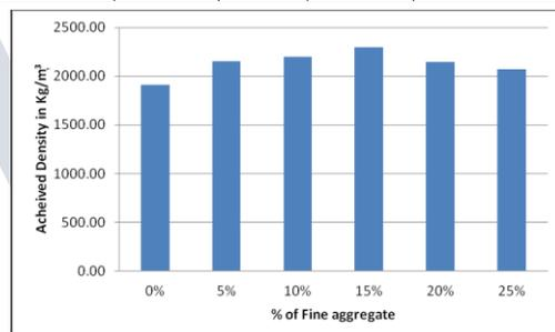
**Fig.6. Percentage fine aggregate and density of PC.**
