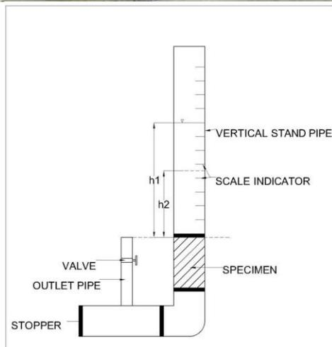
**Fig.5. Permeability testing apparatus.**
