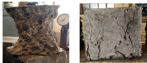
a. Conventional Concrete b. Fiber Reinforced Concrete Fig. 4. Failure Pattern of Cube Compressive Strength
