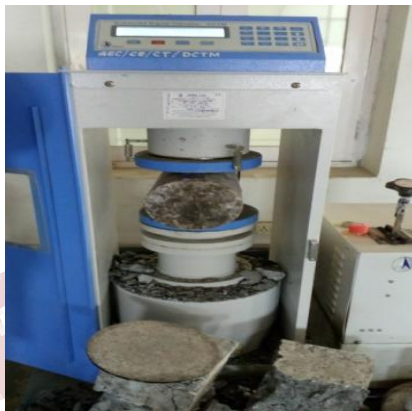
Fig.6 showing cylinder testing
