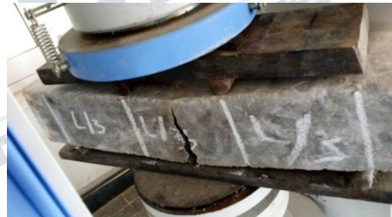
Fig.4 showing Prism testing
