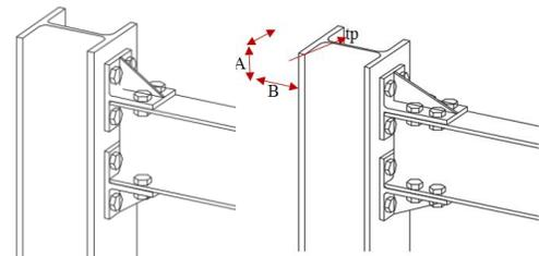
Fig. 1. proposed three-dimensional top and seat T connections
