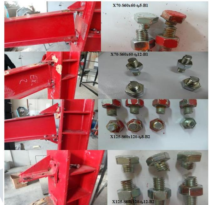
**Fig.4. Failure of models for all models**
