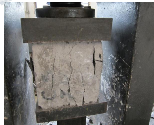
Fig (c) Conventional specimen under compression
