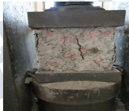
Fig (b) PRFC specimen under compression
