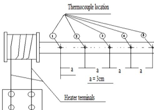
**Fig.1 Cylindrical fin with thermocouple**
