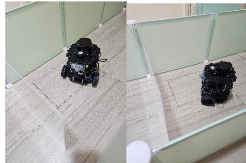
Fig. 8 Avoiding obstacles using the vision-based method
