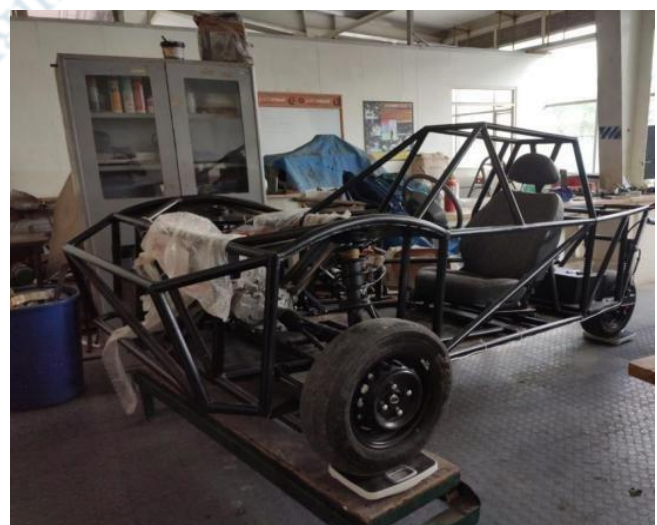
Figure 17. Inclination of Tadpole vehicle for determination of CG Height
