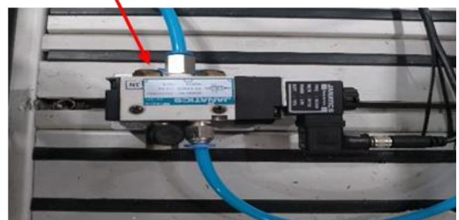
Figure 2(b): Solenoid valve.
