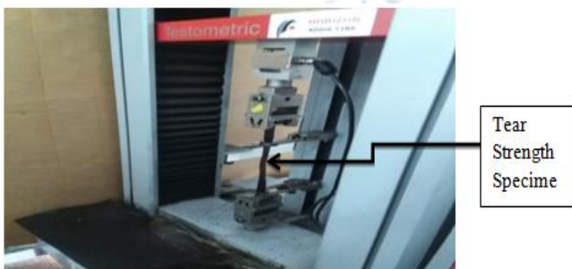
Fig.16: Tear strength testing process using universal tear strength testing machine
