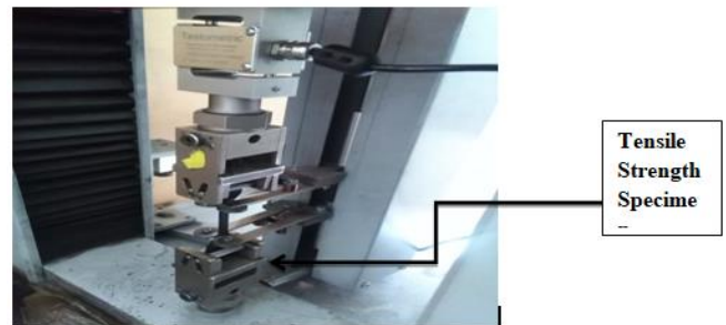
Fig.8: Tensile strength testing process using universal tensile strength testing machine
