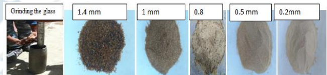
Fig.3: Prepared different sized glass powder/reinforcement
