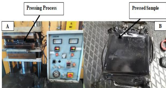
Fig. 6: Pressing process (Fig-A) and Pressed sample (Fig-B)
