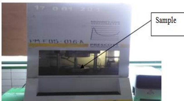
Fig.23: Testing the consistency, compatibility, and sticky property using Mooney line Viscometer
