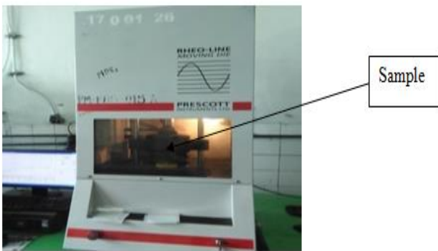
Fig.22: Measuring maximum heat resistance capability using Rheometer
