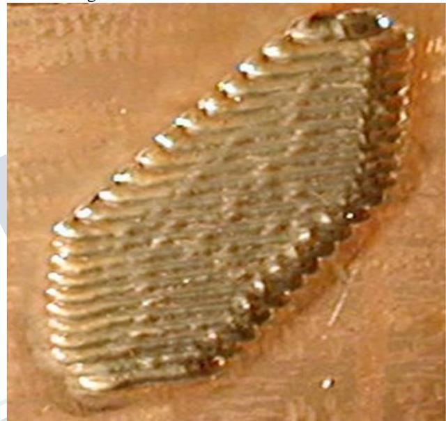
**Figure 8. repair patch complete**
