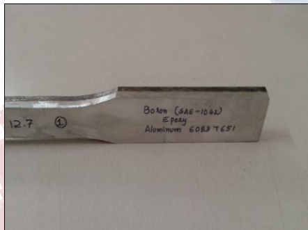
Fig. 2 Before Testing of Boron (SAE-1042) / Epoxy / Aluminum (6082 T651) Laminated Metal Composite (LMC) Tensile Specimen No. 1 of dimension 350x32x12, at Micro, Small and Medium Enterprise (MSME) Testing station (Govt. of India) Govindpura ,Bhopal . India
