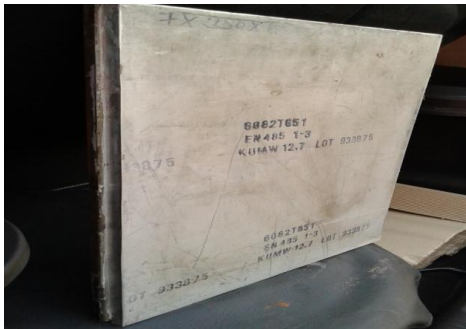
Fig. 1 Laminated Metal Composite (LMC) of Boron (SAE-1042) / Epoxy / Aluminum (6082 T651) of dimensions 450 mm x 380 mm x 24 mm (each metal plate has a thickness of 12 mm), manufactured at M/s Permal Wallace Pvt. Ltd. Bhopal. MP (India)
