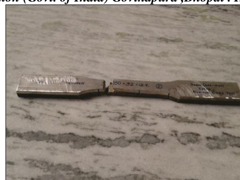
Fig. 6 After Testing of Boron (SAE-1042) / Epoxy / Aluminum (6082 T651) laminated Metal Composite
