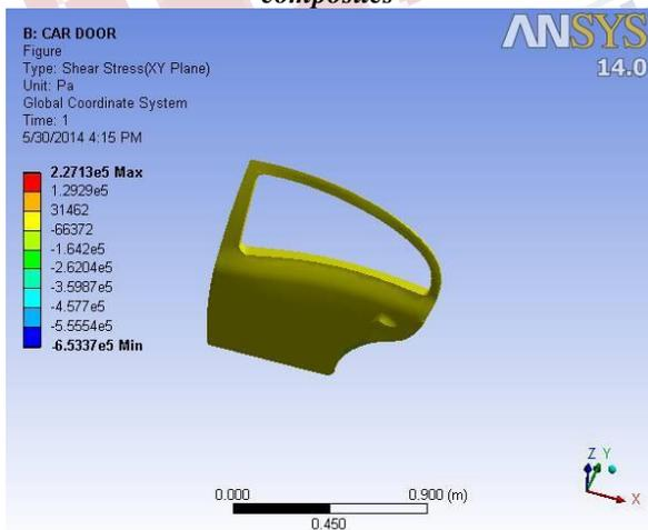
**1.22 Car Door Shear Stress in short fiber Composites**
