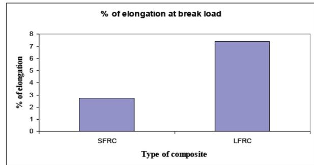
**Fig 1.14: Plot of % elongation at break load v/s type of composite**
