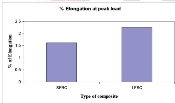
**Fig 1.13: Plot of % elongation at peak load v/s type of composite**
