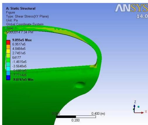
*Fig 1.19 Car Door Shear stress in long fiber composite*
