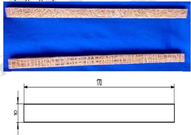
**Fig 1.4: Bending test specimen**
