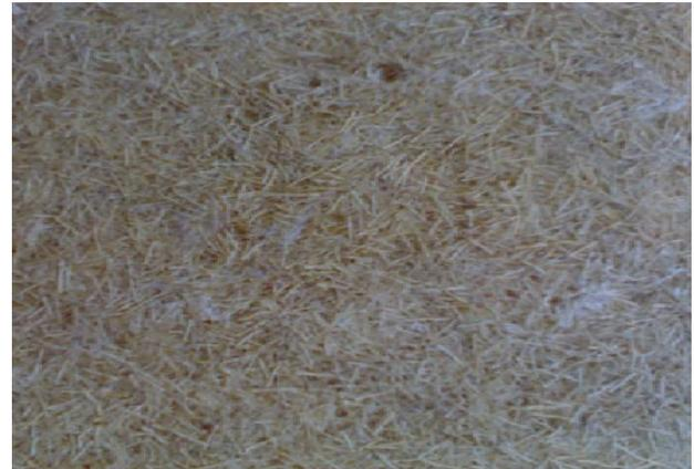
**Fig 1.3(b): Short waived sisal fiber reinforced composite**
