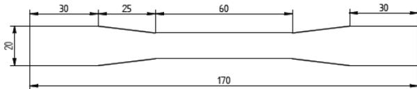
**Fig 1.5: Tensile test specimen**
