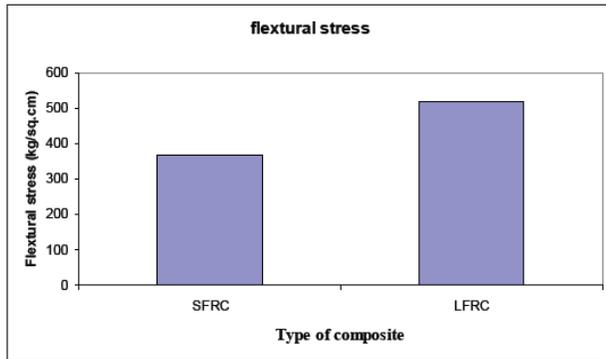
**Fig 1.12: Plot of flextural stress v/s type of composite**
