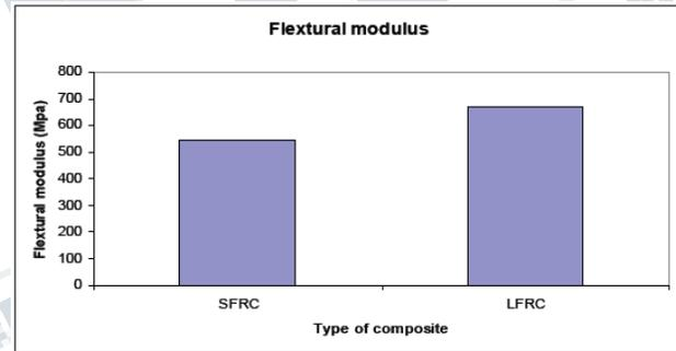
**Fig. 1.15: Plot of flextural modulus v/s type of composite**
