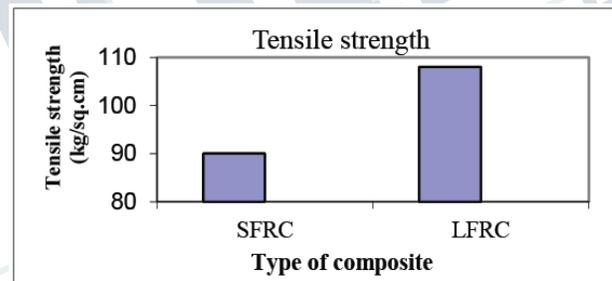
Fig 1.9: Plot of tensile strength v/s type of composite
