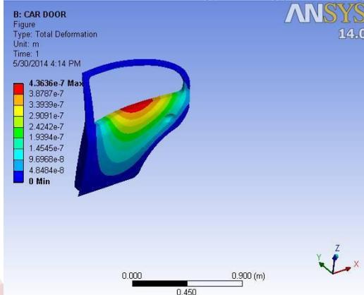
**1.21 Car Door Total Deformation in short fiber composites**
