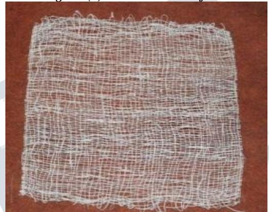
**Fig 1.2(b): Prepared sisal fiber woven Fabric**
