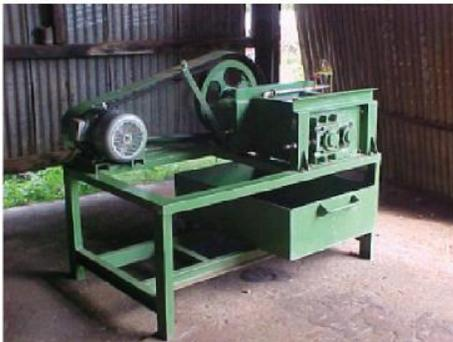
**Fig 1.1(b): Fiber extracting machine**
