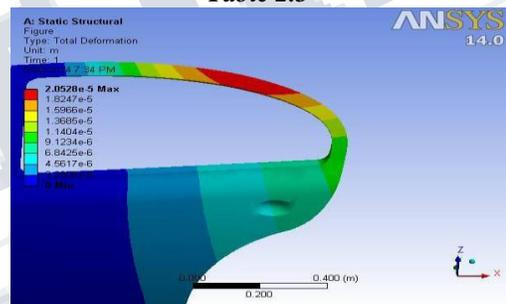
*Fig 1.18 Car Door Total Deformation in Long fiber composite*
