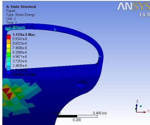
**Fig 1.20 Car Door Strain Energy in long fiber composite**
