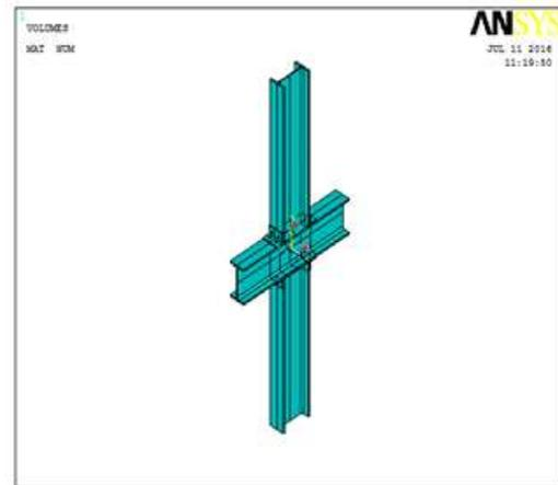
*Fig.7. Ansys model of unstiffened connection*
