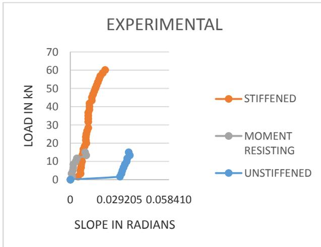
*Fig 7 load versus slope curve*
