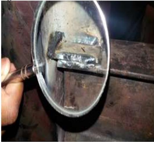
**Fig.4. Failure of stiffened seated connection**
