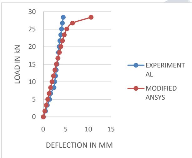
Fig.10. Load versus deflection curve
