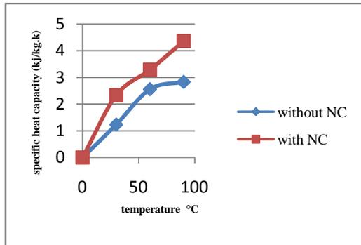
**Graph-2: shows comparison of specific heat capacity of composite with and without Nano carbon.**
