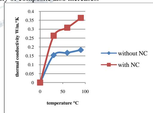
**Graph-1: shows comparison of thermal conductivity of composite with and without Nano carbon.**
