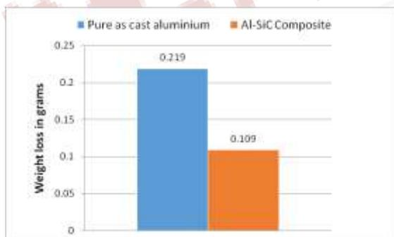
**Figure 9: Comparison of total weight loss at a load of 30N & disk diameter of 130mm**
