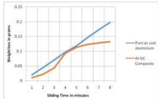
**Figure 4: Comparison of wear behavior at a load of 50N & disk diameter of 100mm**
