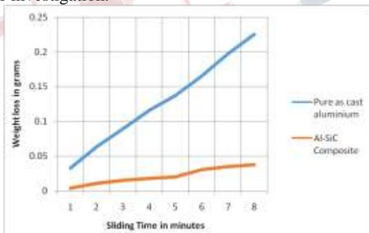
**Figure 3: Comparison of wear behavior at a load of 30N & disk diameter of 100mm**
