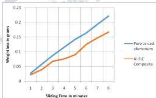
**Figure 6: Comparison of wear behavior at a load of 50N & disk diameter of 130mm**
