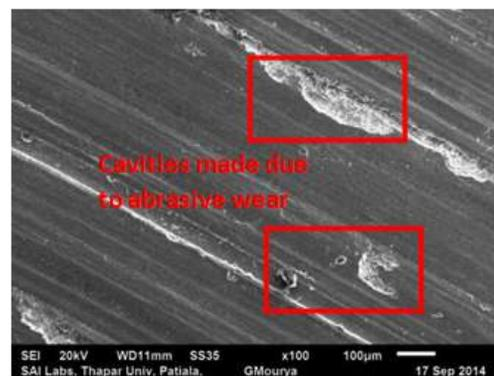
**Figure 11: SEM images of Al-SiC composite at a magnification of 100x**
