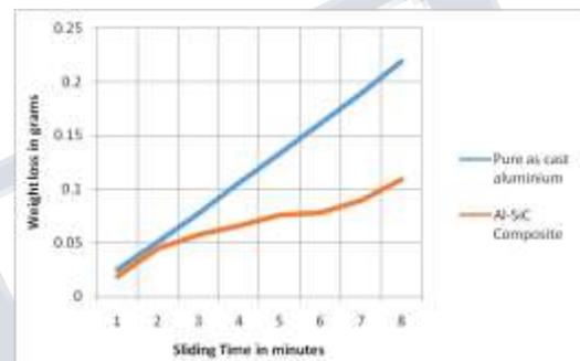
**Figure 5: Comparison of wear behavior at a load of 30N & disk diameter of 130mm**
