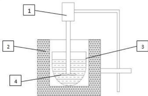
*Figure 1: Stir casting set up*
