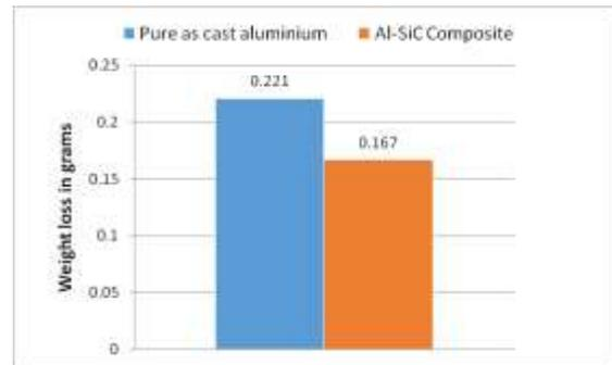
**Figure 10: Comparison of total weight loss at a load of 50N & disk diameter of 130mm**
