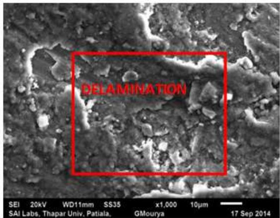
**Figure 12: SEM images of Al-SiC composite at a magnification of 1000x**
