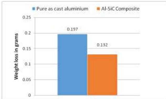
**Figure 8: Comparison of total weight loss at a load of 50N & disk diameter of 100mm**
