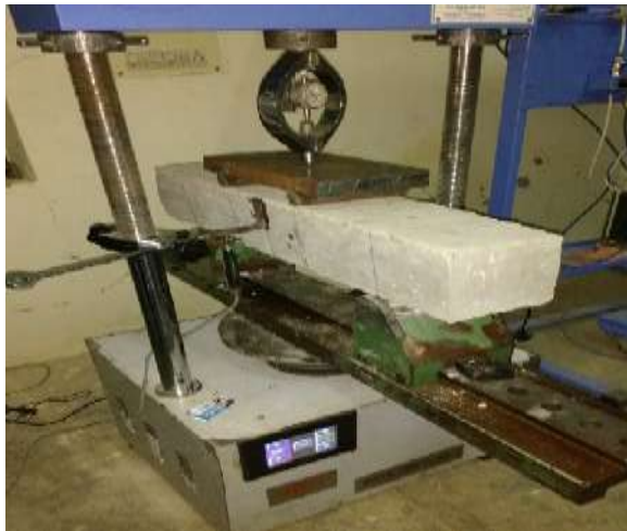
Fig 2: Set up for the evaluation of flexural strength and load- deflection plot
