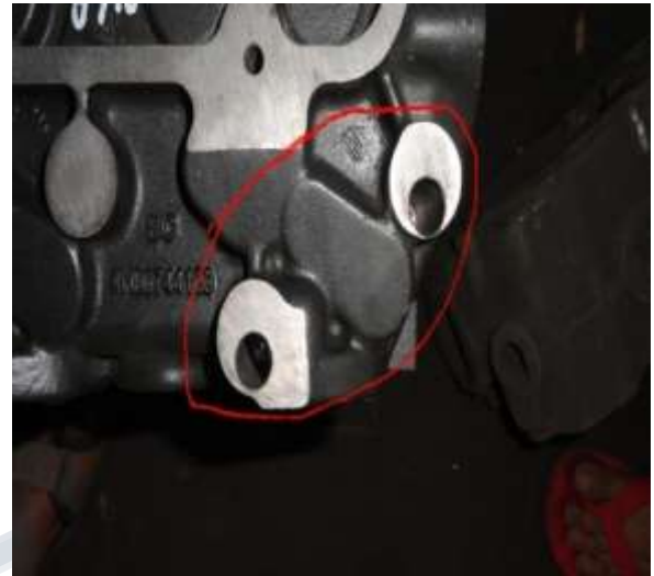
Fig.2 Oversize of bore
