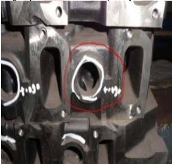
Fig.1 Cylinder Head Dowel Shift and patch mark
