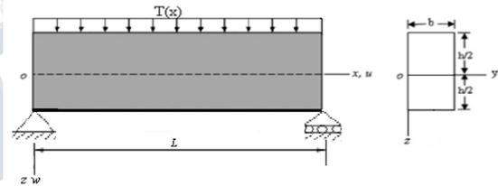
Figure 1: Simply supported beam bending under  $x$ - $z$  plane
