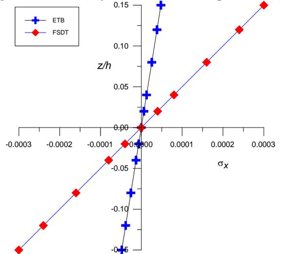
**Figure 4: Variation of Maximum Axial Stress ( $\sigma_x$ )**
