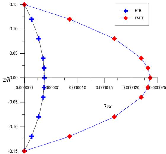
**Figure 5: Variation of Maximum Transverse Shear Stress ( $\tau_{xz}$ )**
