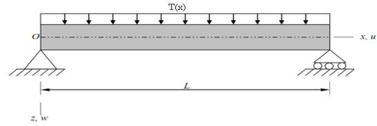
Figure 2: A simply supported uniform beam subjected to thermal load
