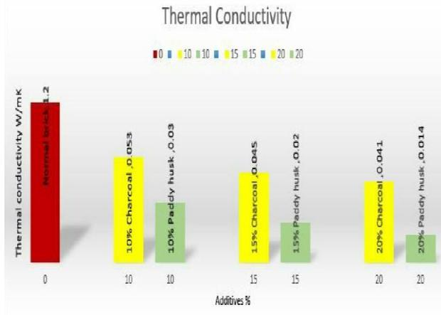
**Fig 7 Additive % vs Thermal Conductivity**
