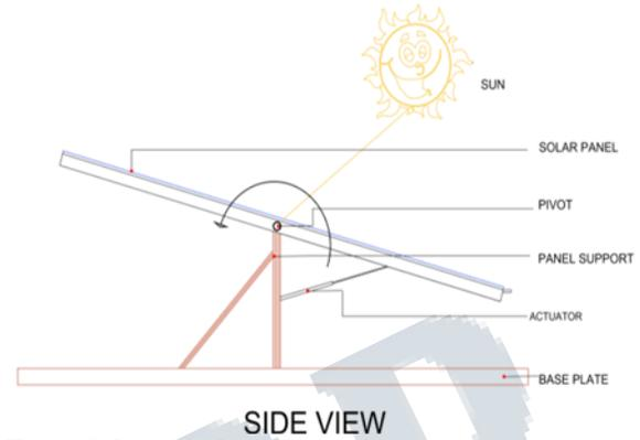
**Fig.4. Solar panel and linear actuator arrangement**
