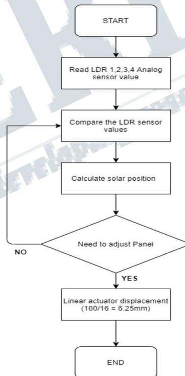
**Fig.2. Algorithm of Solar Tracking System.**
