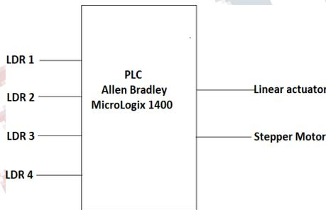
**Fig.3. Input/Output ports of PLC.**
