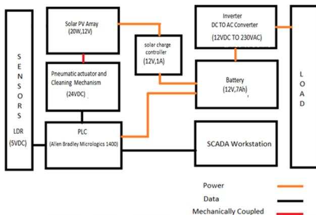
**Fig.1. Block Diagram of Solar Tracking System.**
