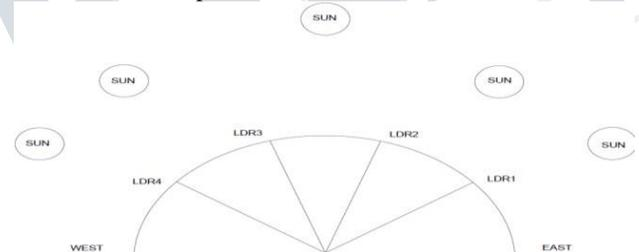
**Fig.6. LDR Positioning on hemispherical solid**
