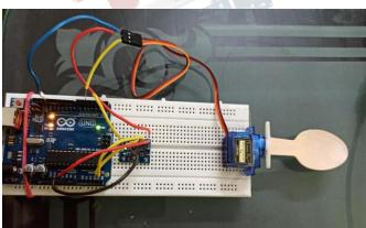
Fig. 6 The resulting prototype of the proposed spoon
