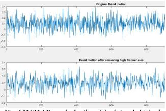
Fig. 4 MATLAB graphs for the original signal obtained and with the high frequencies removed.
