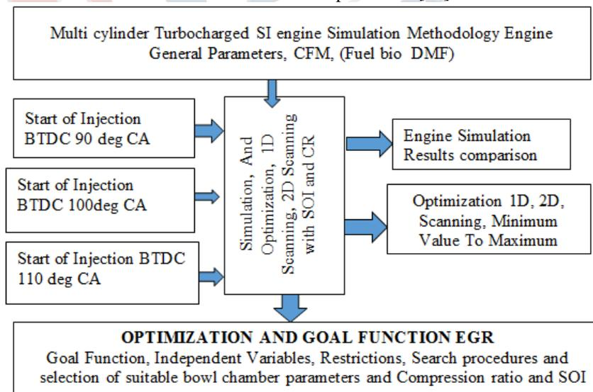
Figure 2.1 Diesel RK simulation methodology for Multi-cylinder DMF engine
