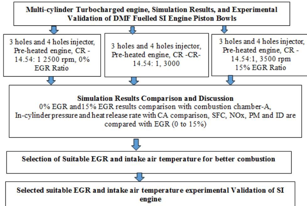
Figure 2.2 Multi-cylinder pre-cooled turbocharged engine simulation methodology
