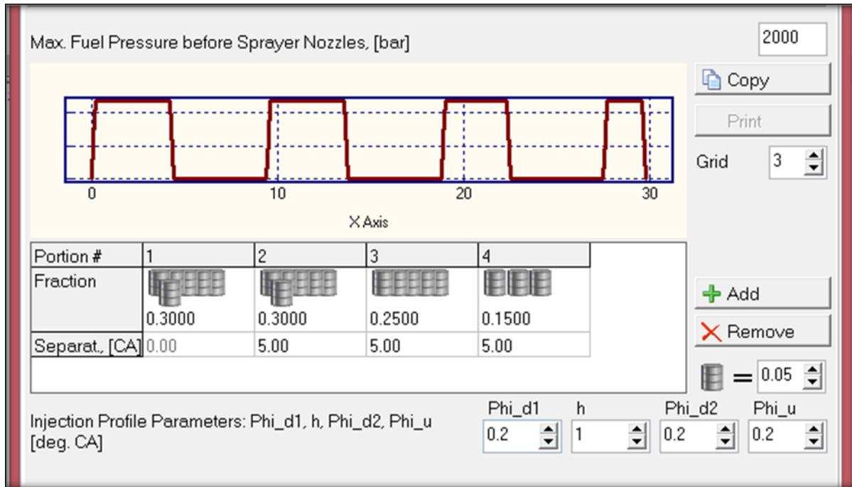
**Figure 2.8 Fuel Injection and profile parameters**
