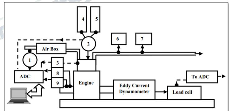
Airflow sensor, 2. Fuel flow sensor, 3. A pressure sensor, 4. Diesel tank, 5.DMF tank, 6. Five gas analysers, 7. Smoke Meter, 8. RPM Indicator, 9. Crank Angle encoder.
