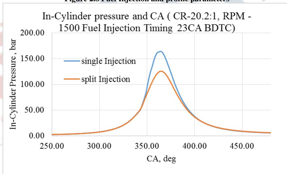
**Figure 2.9 In-Cylinder Pressure Vs CA of single and split injection**
