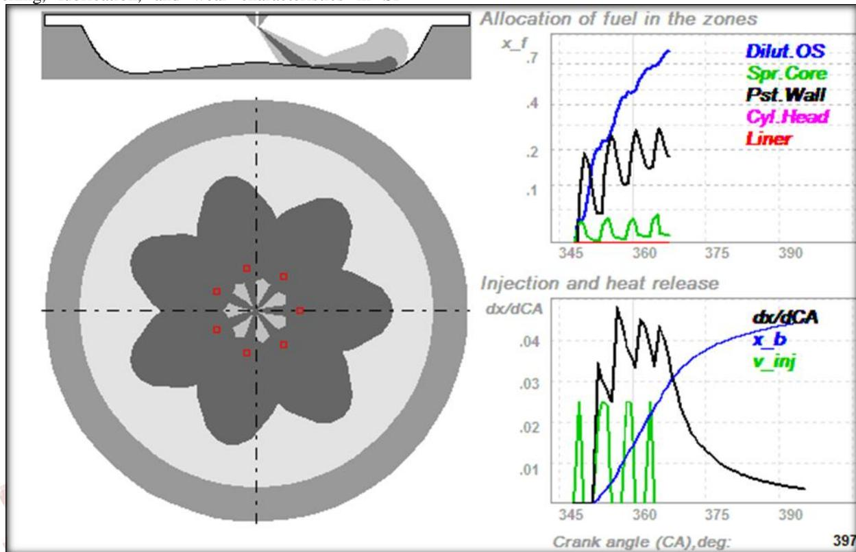
**Figure 2.10 Allocation of fuel in the zones and injection profile and heat release rate Vs CA of split injection**
