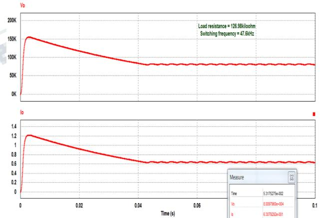
**Fig-10.1(b)** output voltage waveform for load resistance value 126.98kΩ
