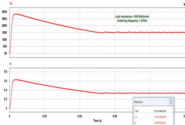
**Fig-10.1(c) Output waveform for load resistance value 454.54kΩ.**
