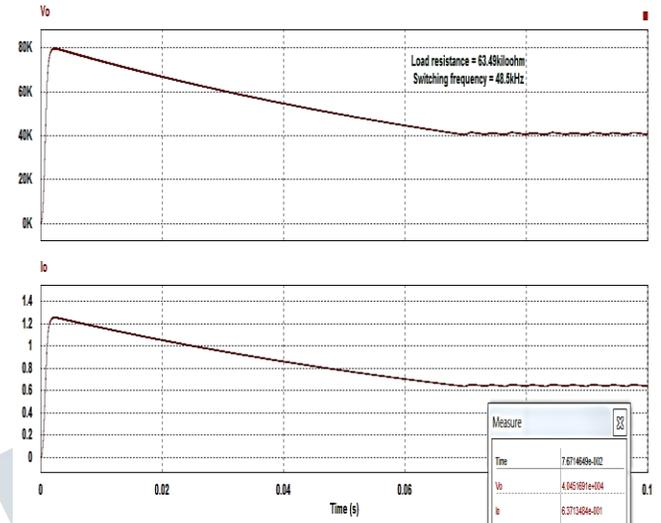
**Fig-10.1(a)** output voltage waveform for load resistance value 63.49kΩ
