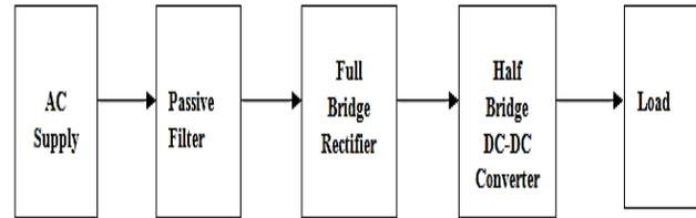
**Fig-3.3 Block diagram of LLCCLL filter with half bridge dc-dc converter.**
