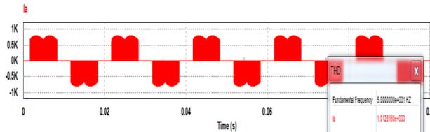
**Fig-9.1** Input current waveform.
