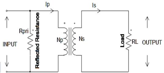
*Fig-6.1 Connection of reflected resistance at primary side of the transformer.*
