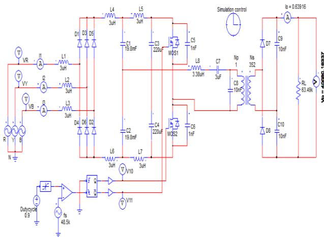
**Fig-8.1** circuit diagram of LLCCLL filter design with bridge rectifier, half bridge dc-dc c0nverter and load.
