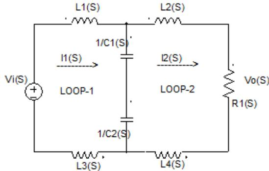
*Fig-5.1 shows the LLCCLL filter system model.*
