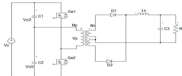
**Fig-3.1 Isolated half bridge dc-dc converter.**
