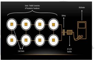
FIG.3 SERIES PARALLEL CONNECTIONS OF PIEZOELECTRIC DISCS[7]
