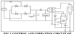
FIG.3 CONTROL AND VIBRATION CIRCUIT OF SYSTEM[5]
