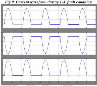
Fig 10. Current waveform during L-L fault condition.
