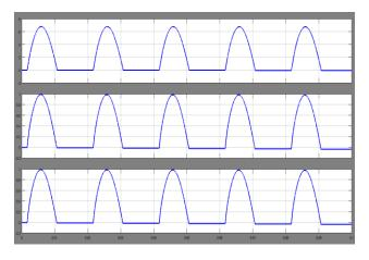
Fig 8. Current waveform during L-G fault condition
