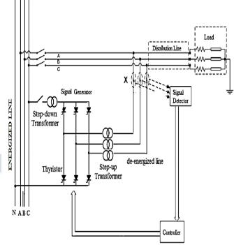
Fig. 3. Three-phase thyristor bridge-based fault detection scheme.
