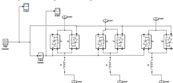
**Fig.1 Thyristor Switched Reactor.**
