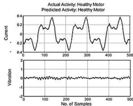
**Figure 5: Results of fault detection and isolation for healthy motor condition**
