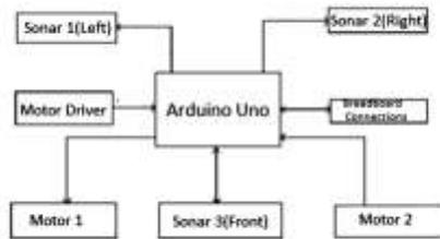
**Fig.2. Overall Block Diagram**
