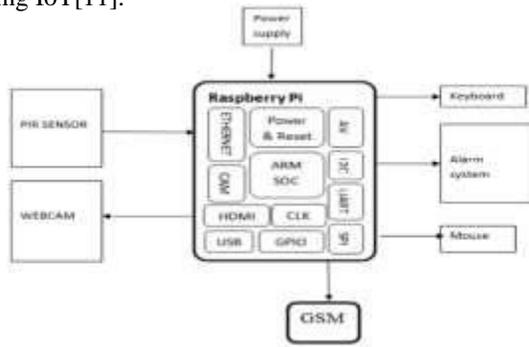
**Fig 5. Block Diagram of Motion Detection and Alarm System**
