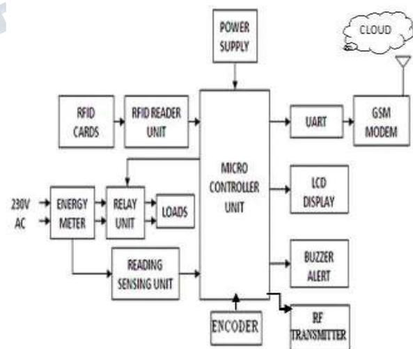
*Fig: 1 Proposed block diagram of Transmitter*
