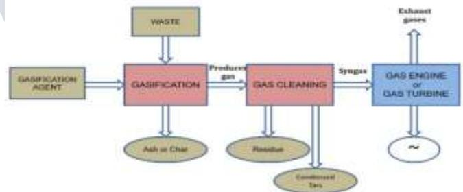
**Fig. 3. Schematic arrangement of the gasification-based configurations of power gasifier**
