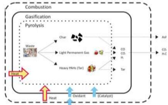
**Fig. 2. Schematic representation of pyrolysis, gasification and combustion stages**
