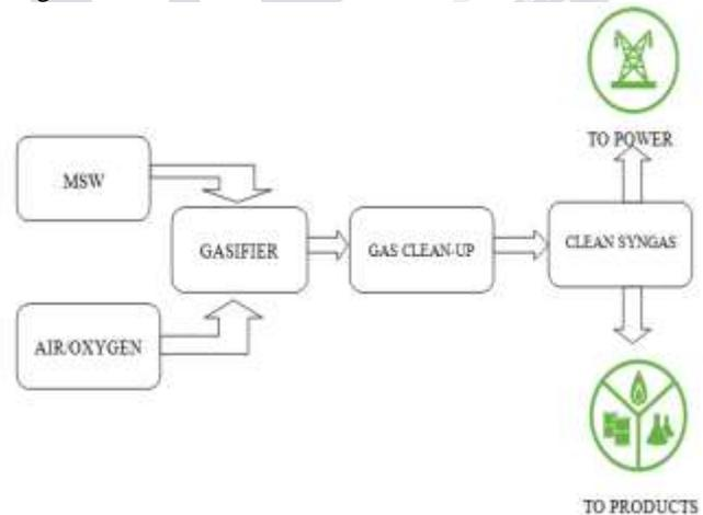
*Fig.1 Gasification process*
